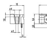
The pin strip 120-M-217, with fastening flanges and a pitch of 5 mm, is available in 2- to 12-pole design and can be mounted side-by-side.
