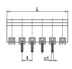
The pin strip 120-M-227, with connecting flanges and a pitch of 5 mm, is available in 2- to 12-pole design and can be mounted side-by-side.
