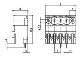
The pin strip 120-M-285, tall version with connecting flanges and a pitch of 5 mm, is available in 2- to 12-pole design and can be mounted side-by-side.
