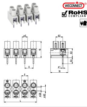
The plug-in terminal strip 302-FBG is equipped with a solder pin and designed for the use on PCBs. Due to the small 8 mm pitch, this design is well suited for applications where space is limited.
