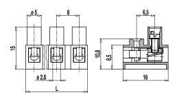
The plug-in terminal strip 302-FLW-DS in 8 mm pitch is available with 2 to 12
