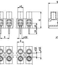
The socket terminal strip 302-G is one of our smallest socket terminal strips. It is available in 8 mm pitch with 2- to 12-pole design and can be easily stripped to the desired number of poles.
