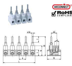
The plug-in terminal strip 302-NSLP, low version, is available in 8 mm pitch with 2 to 12 poles.
