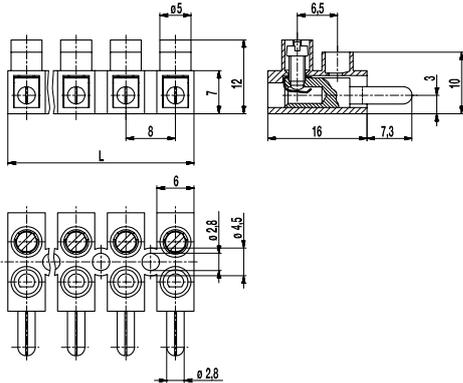
The plug-in terminal strip 302-NSTS, lower version, is available in 8 mm pitch with 2 to 12 poles.
