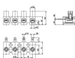
The tab connector block 322-A-2,8 in 10 mm pitch is available with 1 to 12 poles. These connector strips are a combination of screw and tab connectors. The can be used to connect equipment to the grid and are well suited for many other applications.
