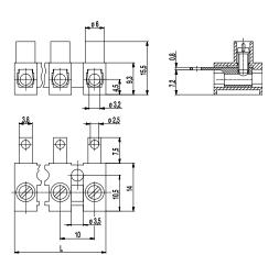
The screw/solder terminal strip 322-LFS in 10 mm pitch was designed for larger cross-sections than version 302-LF-DS. It is available with 1 to 12 poles. Mouldings of this type are open on the solder tag side but they can be connected safe-to-touch as 2- and 3-pole version with cover caps A-323 and base plates B-323. This will extend the creepage distance to the mounting surface. Socket and solder tag are manufactured in one piece.
