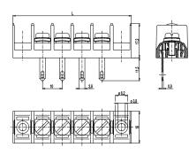
Screw/solder connector block 983-ML-2,8 in 10 mm pitch is available in 2- to 12-pole design and can be mounted side-by-side in nominal pitch. This connector is based on our series 983 terminal strip.
