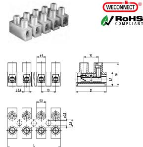
The plug-in terminal strip 323-FB is available in 10 mm pitch with 2 to 12 poles. It has one screw connection per pole and one plug connection for a terminal strip with pins.
