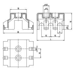
Cover caps A-323 are combined with base plates B-323 in order to ensure a safe-to-touch protection of the socket strip.
