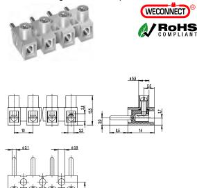
The 322-D-SV is based on our established plug-in terminal strip 322-SV. The clamping space is enlarged for 2x2,5 mm<sup>2</sup> solid wire without wire protector or 2x1,5 mm<sup>2</sup> with wire protector. Therefore, this version is most suitable when connections of two wires per pole are required.
