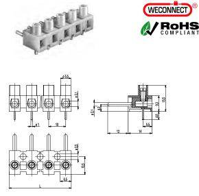
The plug-in terminal strip 322-SVG with a pitch of 10 mm is equipped with a solder pin and designed for the use on PCBs. Due to large pitch and moulding shape, this version is also well suited for applications using higher voltages.
