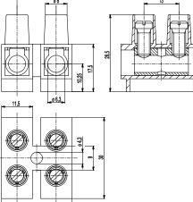
The socket terminal strip 327-FU with raised base and a pitch of 14,5 mm is available in 1 to 12 pole design.
