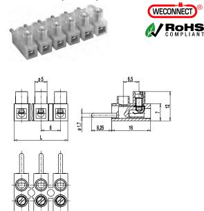
The plug-in terminal strip 302-NSV, lower version, is available in 8 mm pitch with 2 to 12 poles.
