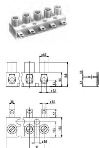
The screw/solder terminal strip 321-LFS in 10 mm pitch was designed for larger cross-sections than version 302-LF-DS. It is available with 1 to 12 poles. Mouldings of this type are encapsulated on the solder tag side and therefore particularly well suited for potting.
