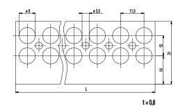
Marking strips BST-324 for our 324 series terminal strips are available in 2- to 12-pole and in 56-pole design (length: 643,50 mm). The customer can strip them easily to the desired pole number.
