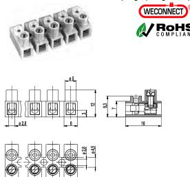
The plug-in terminal strip 302-NFLW-DS, low version, is available in 8 mm pitch with 2 to 12 poles.
