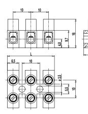
The socket terminal strip 323 is available in 10 mm pitch with 1- to 12-pole design and can be easily stripped to the desired number of poles.
