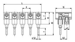
The plug-in terminal strip 302-NSLP, low version, is available in 8 mm pitch with 2 to 12 poles.
