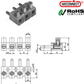
The plug-in terminal strip 322-STFS is available in 10 mm pitch with 2 to 12 poles. It has one screw connection per pole and one vertical pin for the connection to the socket of the female counterpart.
