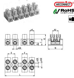
The socket terminal strip 302-N, low version in 8 mm pitch, is available with 1 to 12 poles.
