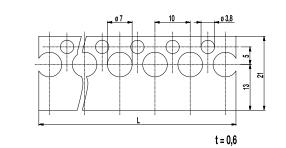
Marking strips BST-322 for our 322 series terminal strips are available in 2- to 12-pole and in 65-pole design (length: 650 mm). The customer can strip them easily to the desired pole number.
