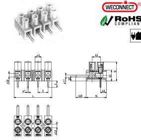
The plug-in terminal strip 302-SVG is equipped with a solder pin and designed for the use on PCBs. Due to the small 8 mm pitch, this design is well suited for applications where space is limited.
