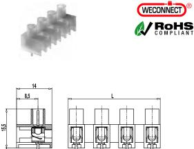
The plug-in terminal strip 322-FBG with a pitch of 10 mm is equipped with a solder pin and designed for the use on PCBs. Due to large pitch and moulding shape, this version is also well suited for applications using higher voltages.
