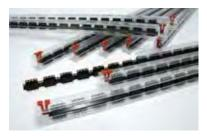
Our 550 mm bar magazines have various geometries which are tailored to the individual component size and shape. Both magazine ends are closed with a plug that is easy to remove.
