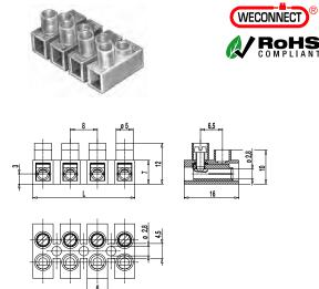
The plug-in terminal strip 302-NSTB, lower version, is available in 8 mm pitch with 2 to 12 poles.
