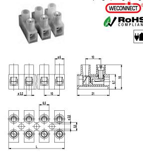
The plug-in terminal strip 323-FBW is available in 10 mm pitch with 2 to 12 poles. It has one screw connection per pole and one plug connection pointing upwards for the connection of a terminal strip with pins.
