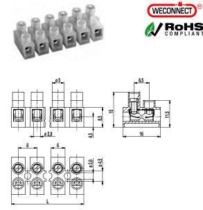
The plug-in connector strip 302-FB is available in 8 mm pitch with 2 to 12 poles. It is well suited for applications where space is limited.
