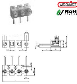
The plug-in terminal strip 322-SVW is available in 10 mm pitch with 2 to 12 poles. It has one screw connection per pole and one vertical pin for the connection to the socket of the female counterpart.
