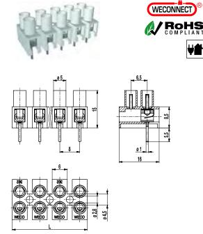
The plug-in terminal strip 302-FBG is equipped with a solder pin and designed for the use on PCBs. Due to the small 8 mm pitch, this design is well suited for applications where space is limited.
