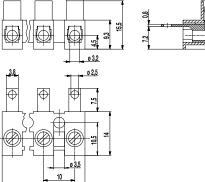
The screw/solder terminal strip 322-LFS in 10 mm pitch was designed for larger cross-sections than version 302-LF-DS. It is available with 1 to 12 poles. Mouldings of this type are open on the solder tag side but they can be connected safe-to-touch as 2- and 3-pole version with cover caps A-323 and base plates B-323. This will extend the creepage distance to the mounting surface. Socket and solder tag are manufactured in one piece.
