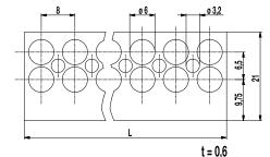
Marking strips BST-302 for our 302 series terminal strips are available in 2- to 12-pole and in 81-pole design (length: 648 mm). The customer can strip them easily to the desired pole number.
