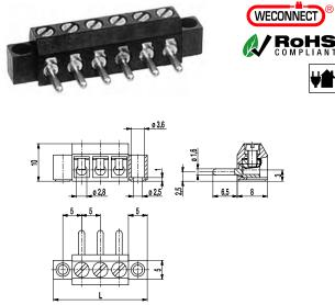
The plug-in connector strip 951-B-SV in 5 mm pitch is available with 2 to 12 poles. Contrary to version 951-SV, the plug connector 951-B-SV has exterior mounting flanges and can be used in combination with version 971-FBS.
