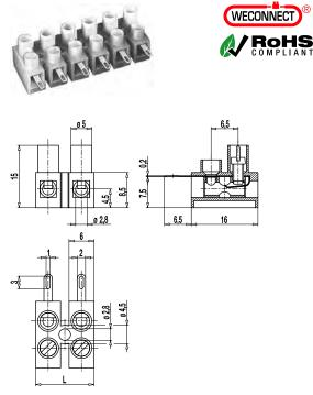
The screw/solder terminal strip 302-LF-DS in 8 mm pitch is available with 1 to 12 poles. Due to the small pole spacing, it is well suited for applications where space is limited.
