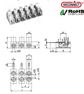
The screw/solder terminal strip 302-NLF-DS, lower version, is available in 8 mm pitch with 1 to 12 poles.
