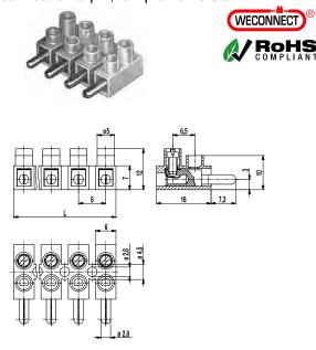
The plug-in terminal strip 302-NSTS, lower version, is available in 8 mm pitch with 2 to 12 poles.
