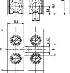
The socket terminal strip 326 is available in 14,5 mm pitch with 1- to 12-pole design and can be easily stripped to the desired number of poles. This version has a large terminal space and a creepage distance of more than 7 mm measured from terminal body to mounting surface. That is why this terminal strip is suitable for voltages up to 750 V.
