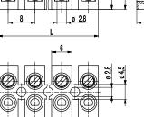
The plug-in terminal strip 302-STB is available in 8 mm pitch with 1 to 12 poles. It has one screw connection per pole and one plug connection for a terminal strip with pins.
