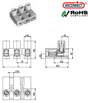
The plug-in terminal strip 321-B is available in 10 mm pitch with 1 to 12 poles. It has one screw connection per pole and one plug connection for a terminal strip with pins.
