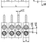
The plug-in terminal strip 302-SV is available in 8 mm pitch with 1 to 12 poles. It has one screw connection per pole and one vertical pin for the connection to the socket of the female counterpart.
