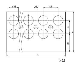
Marking strips BST-327 for our 326 and 327 series terminal strips are available in 2- to 12-pole and in 44-pole design (length: 638 mm). The customer can strip them easily to the desired pole number.
