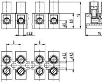
The socket terminal strip 302 is one of our smallest socket terminal strips. It is available in 8 mm pitch with 1- to 12-pole design and can be easily cut to the desired number of poles.
