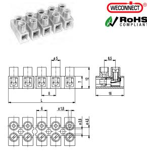
The plug-in terminal strip 302-NFLP-DS, low version, is available in 8 mm pitch with 2 to 12 poles.
