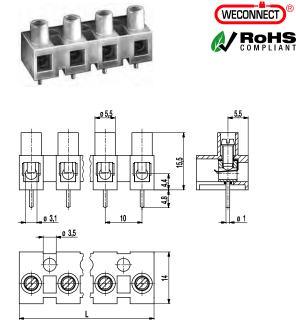
The socket terminal strip 322-G is available in 10 mm pitch with 1- to 12-pole design and can be easily stripped to the desired number of poles. The flexible polyamide moulding can even be mounted on curved surfaces.
