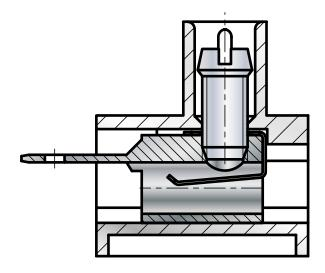
Tab and screw connector blocks are a combination of screw terminals and tab connector blocks.
