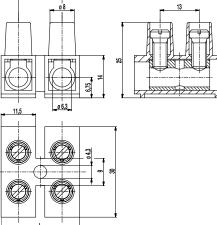
The socket terminal strip 327 is available in 14,5 mm pitch with 1- to 12-pole design and can be easily stripped to the desired number of poles.
