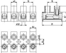
The plug-in terminal strip 323-STFB is available in 10 mm pitch with 2 to 12 poles. It has one screw connection per pole and one plug connection for a terminal strip with pins.
