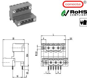
The pin strip 120-M-255, two-tier version with connecting flanges and a pitch of 5 mm, is available in 4- to 24-pole design and can be mounted side-by-side.
