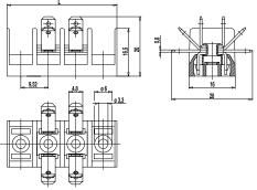
Tab/screw connector block 982-F in 9,52 mm pitch is based on our proven 98.. series (see Catalogue 4 "Pitch 7,5 mm").
