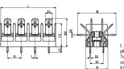
L = Number of poles x pitch Terminal design with tab connector package 8.033
