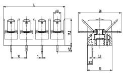
L = Number of poles x pitch Terminal design with tab connector package 8.022
