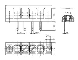
Tab/screw connector blocks 983-MF-2,8 and 983-MF-4,8 in 10 mm pitch are available in 2- to 12-pole design and can be mounted side-by-side in nominal pitch. These connectors are based on our series 983 terminal strips.
